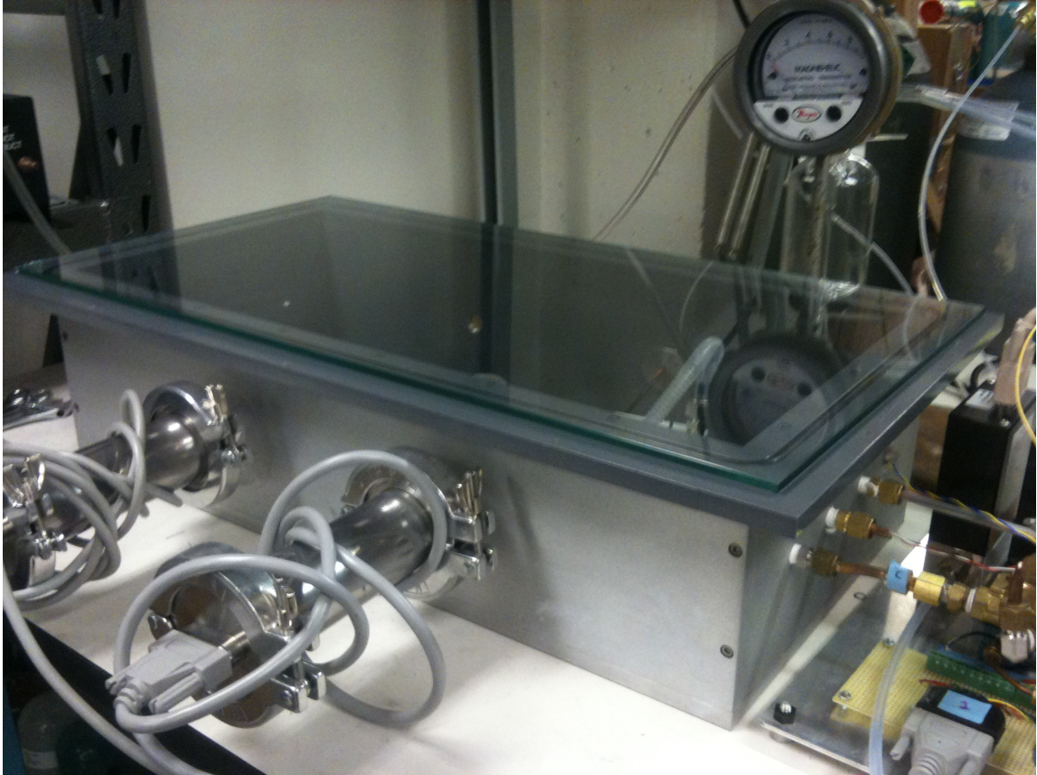
Figure 3.4: Calibration chamber used for sensor drift experiments. mation algorithm we propose.
