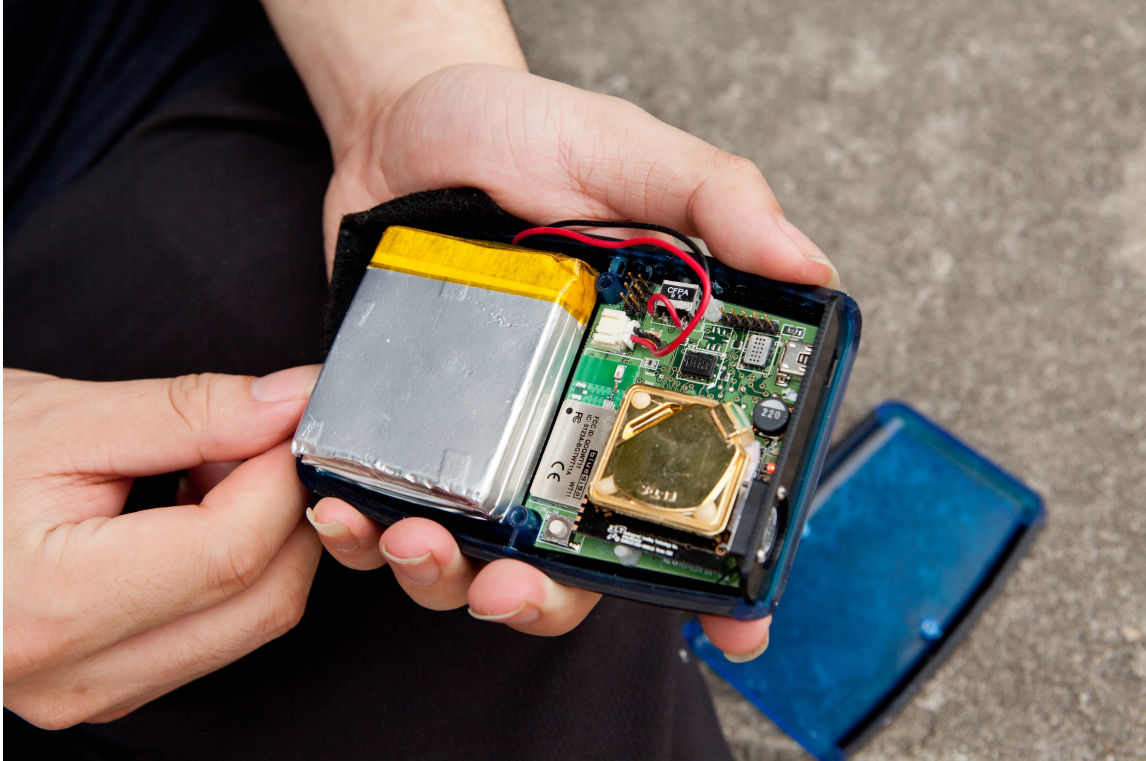
Figure 2.1: M-pod personal air quality sensor.
