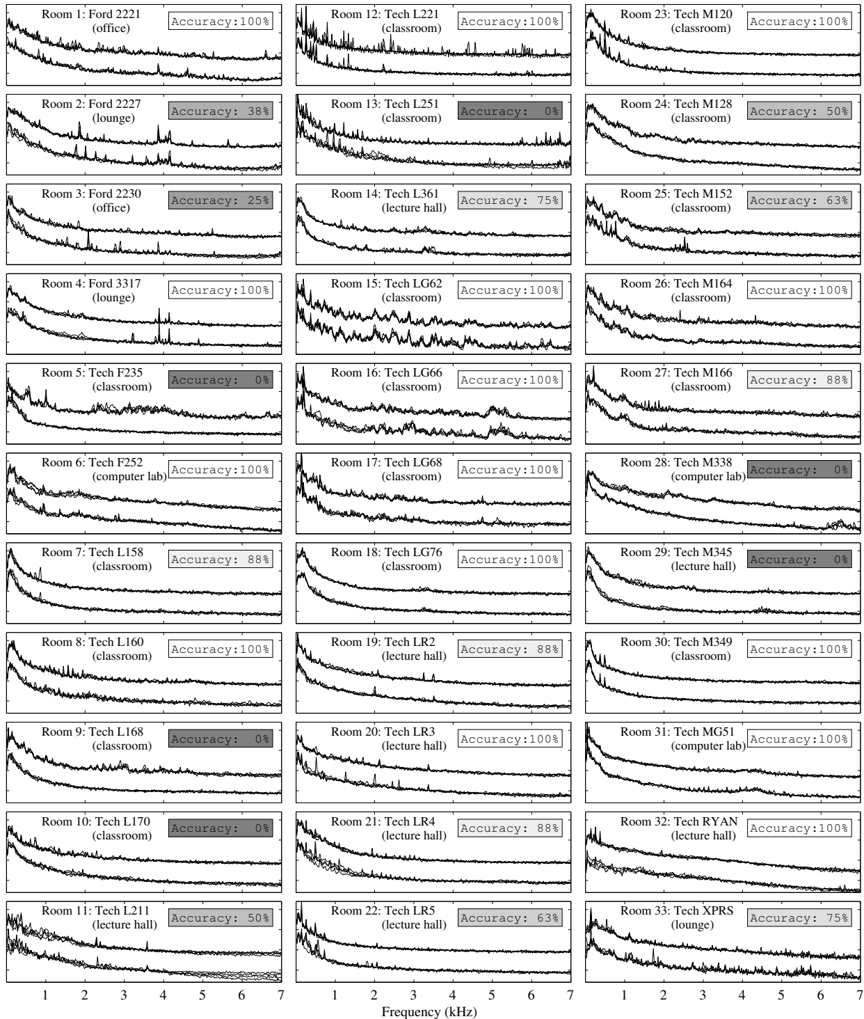
Figure 4.5: Acoustic Background Spectra (ABS) from 33 rooms, using the optimal parameter values. The vertical axis is the ABS value for each frequency bin; these values correspond to the log-scaled power spectrum. Fingerprints from two visits are vertically offset from each other to aid visual comparison. Each visit includes four overlaid fingerprints from different locations within the room.
