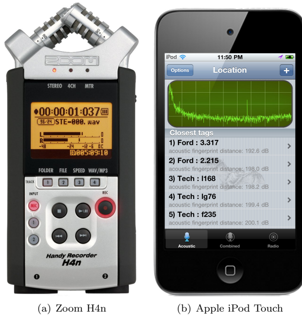
Figure 4.3: Experimental platforms. (a) The Zoom H4n handheld recorder was used to collect traces used in the simulations. Its price is \sim \$300. (b) The Apple iPod Touch (4th generation) running our Batphone localization software was used for the end-to-end experiment.
