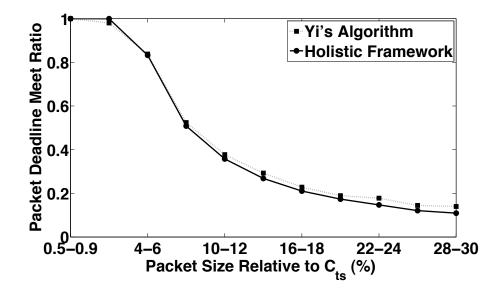
Figure 3.17. Comparison to the work in [114] in terms of packet deadline meet ratio.
