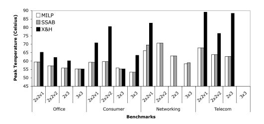
Figure 5.8. Performance comparison between the steady-state analysis based heuristics (based on HotSpot), the MILP, and Xie and Hung's heuristic [111].
