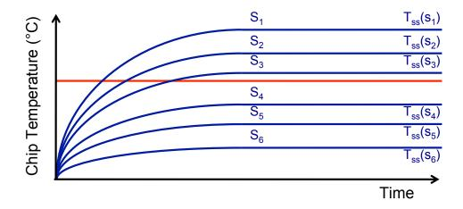
Figure 4.1. The RC curves showing chip temperatures as a function of time due to different speed levels.
