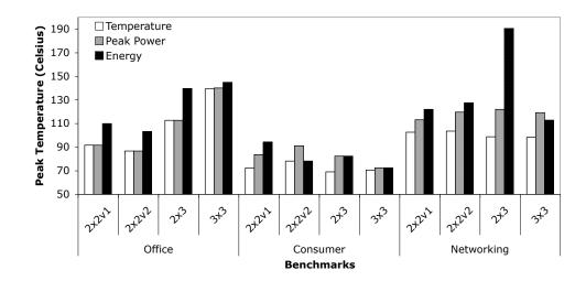
Figure 5.5. Peak temperature minimization vs. energy and peak power minimization for higher power density chips. The results were obtained by solving the MILPs directly. Here, as the chip power density increases, spatial thermal variation becomes significant and peak power minimization is not effective in reducing the chip peak temperature.
