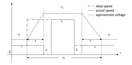
Figure 4.3. Waveforms of speed and voltage levels for two transitions, where S and V denote speed and voltage, respectively. During transitions, the voltage is increased or decreased in a small step size and thus there is a delay associated with each transition.
