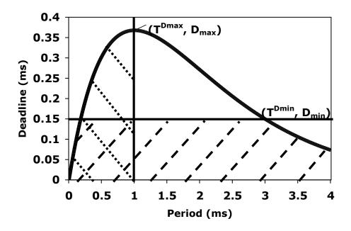
Figure 2.2. Task deadline in milliseconds as a function of task periods, also in milliseconds. The left-slanted and right-slanted areas denote infeasible period and deadline combinations. The unpatterned region represents possibly feasible period and deadline combinations and is where the search process is conducted.
