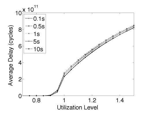
Figure 4.10. Average deadline miss delay (cycles) for different throttling times for the best speed selection policy.
