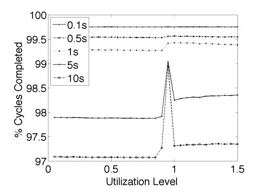
Figure 4.8. Average number of cycles completed (%) for different throttling times for the best speed selection policy.
