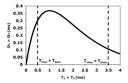
Figure 2.1. Task deadlines in milliseconds as a function of task periods, also in milliseconds. The area inside the vertical dotted lines denotes the acceptable period ranges for the task set in Table 2.1.
