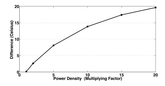
Figure 5.3. Differences in peak temperatures between energy minimization and peak temperature approaches. The x-axis shows the values (i.e., multiplying factors) that were multiplied to the original chip power density. In this example, peak power minimization yields the same peak temperature as energy minimization.
