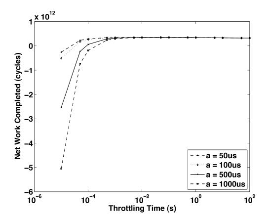
Figure 4.4. Net number of cycles completed as a function of throttling time, where *a* is the voltage changing time from the low speed level to the high speed level. With non-negligible transition overhead, infinitesimally small throttling time does not lead to the maximum amount of work completed.
