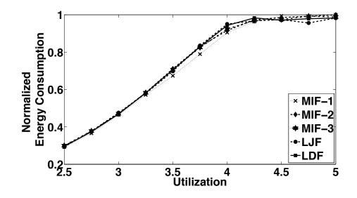
Figure 3.14. Energy consumption of different job assignment algorithms for the four-core case.
