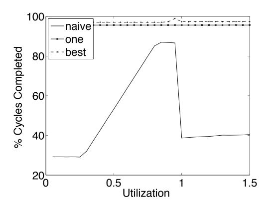
Figure 4.5. Average number of cycles completed (%) for different speed selection policies with throttling time of 10 s.
