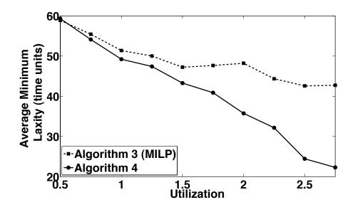
Figure 3.10. Minimum job laxity of different packet scheduling algorithms.
