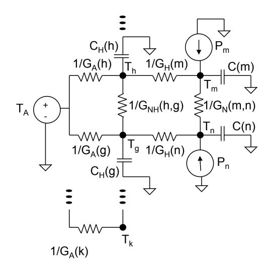
Figure 5.1. Equivalent circuit diagram of the thermal model. In this example, core m is connected to its neighboring core n and is under heatsink element h. The power consumption and capacitance of core m are represented by the current source  $P_m$  and the capacitor C(m), respectively. The heatsink element h is connected to other neighboring heatsink elements, a capacitor, as well as to the ambient, which is denoted by the voltage source  $T_A$ .
