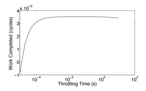
Figure 4.11. Average number of cycles completed as a function of throttling time when transition overhead is considered. A very small throttling time can result in a negative net number of cycles completed.
