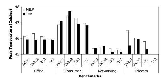
Figure 5.9. Performance comparison between the transient analysis based heuristics (based on HotSpot) and the MILP. Here, the MILP sometimes results in a higher peak temperature because it uses the steady-state thermal analysis, which ignores dynamic thermal effects.
