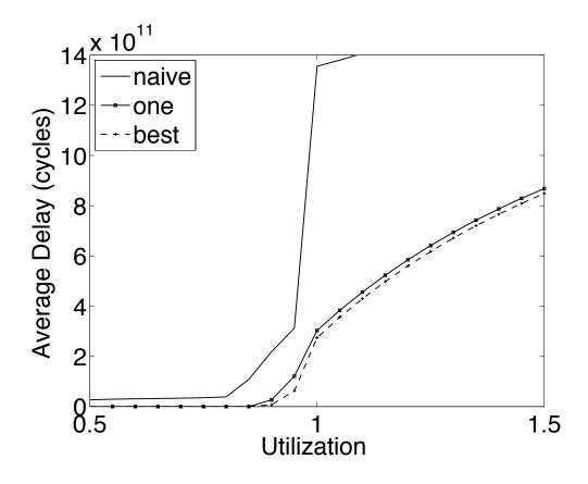
Figure 4.7. Average deadline miss delay (cycles) for different speed selection policies with throttling time of 10 s.
