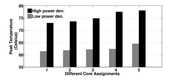
Figure 5.7. Bar plot illustrating the resultant peak temperatures for the different core assignments that can be obtained given the same peak power. The maximum difference in peak temperatures is higher than 5 °C for the Networking benchmark, which contains only 12 tasks.
