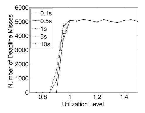
Figure 4.9. Average number of deadline misses for different throttling times for the best speed selection policy.
