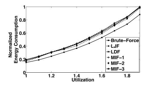
Figure 3.12. Energy consumption of different job assignment algorithms for the two-core case.
