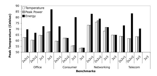
Figure 5.4. Peak temperature minimization vs. energy and peak power minimization. The results were obtained by solving the MILPs directly. Clearly, energy minimization is not effective in reducing the chip peak temperature.
