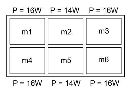
Figure 5.6. An example  $2 \times 3$  floorplan with associated power consumption for each core.
