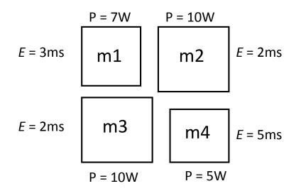
Figure 5.2. Floorplan for the motivating example in Section 5.3, where both task execution times (E) and power consumption (P) are shown for each core.
