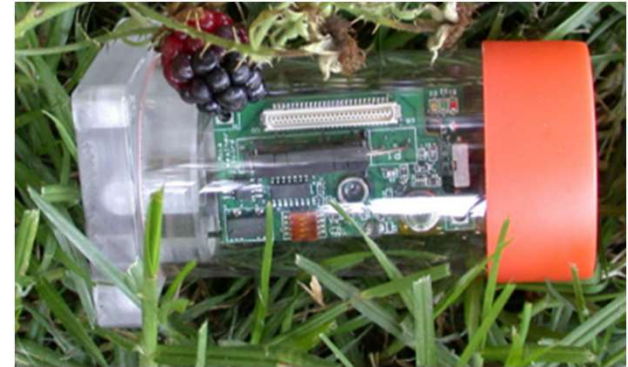
Figure 7: Enclosure for above the ground sensors
