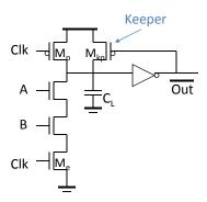
Same approach as level restorer for pass-transistor logic
