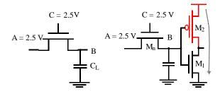
V<sub>B</sub> does not pull up to 2.5V, but 2.5V - V<sub>T</sub>
