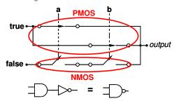
• Basic device in NMOS and PMOS (CMOS) technologies
