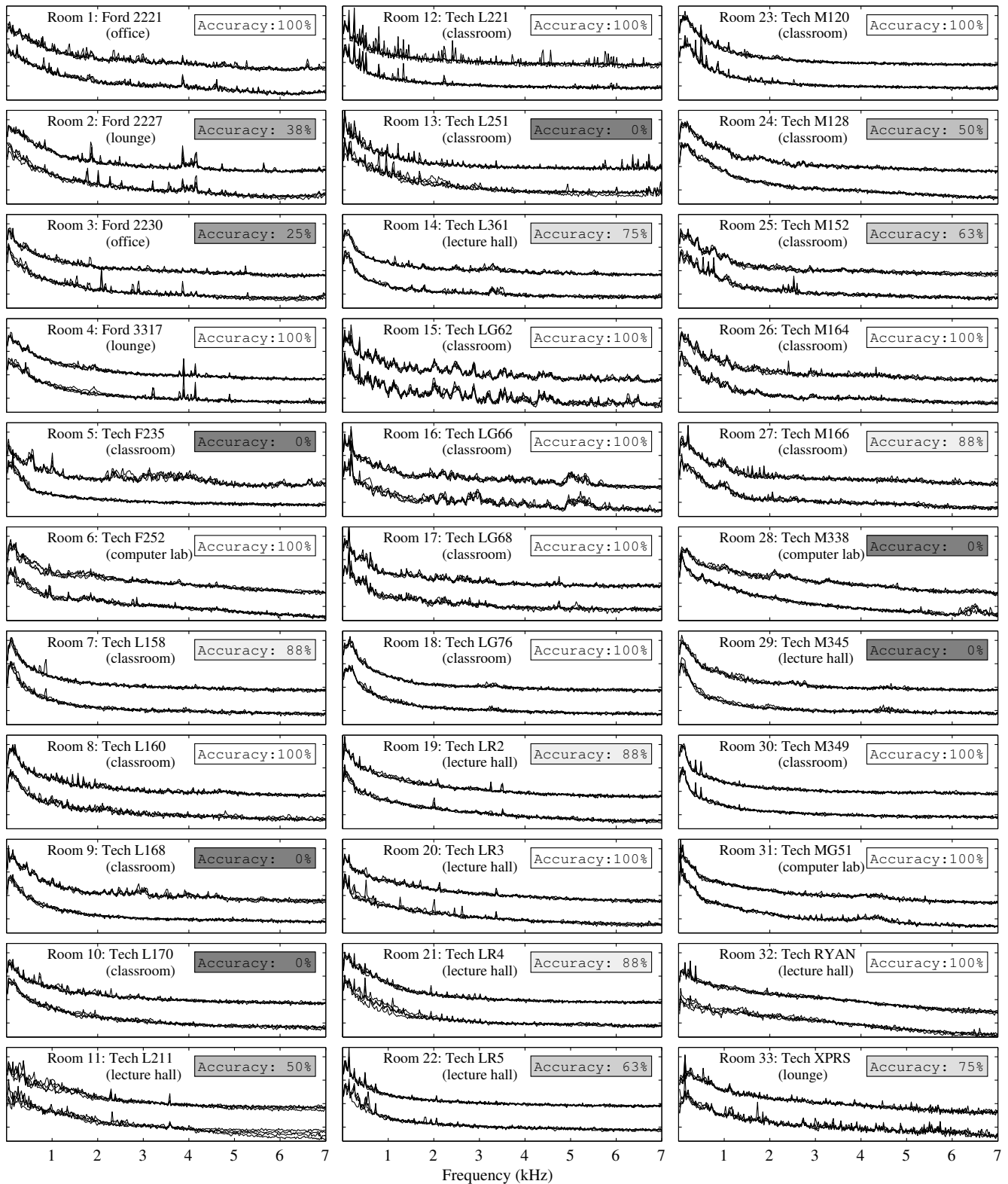
Figure 5: Acoustic Background Spectra (ABS) from 33 rooms, using the optimal parameter values. The vertical axis is the ABS value for each frequency bin; these values correspond to the log-scaled power spectrum. Fingerprints from two visits are vertically offset from each other to aid visual comparison. Each visit includes four overlaid fingerprints from different locations within the room.
