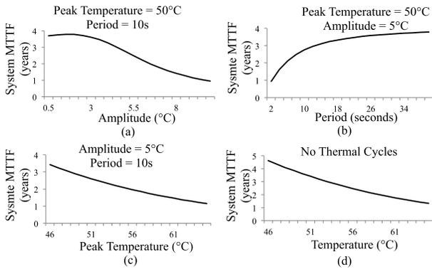
Fig. 1. System MTTF dependence on thermal cycle (a) amplitude, (b) period, and (c) peak temperature, and on (d) temperature without thermal cycles.
