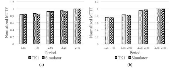
Fig. 7. Normalized MTTFs with TK1 and constructed simulator with (a) frame-based tasks and (b) tasks with random periods.
