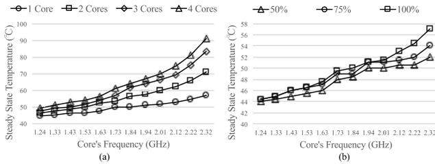
Fig. 5. Steady-state temperature with (a) different numbers of fully loaded cores running at different frequencies and (b) one core running at different frequencies and utilizations.
