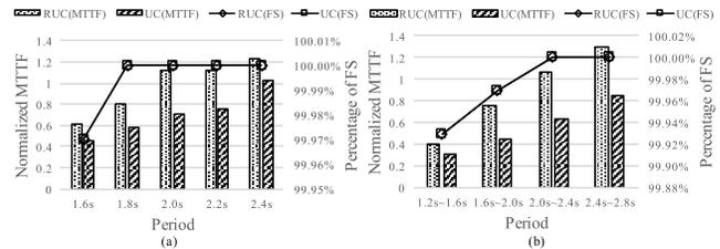
Fig. 12. Normalized MTTF and percentage of FS when running on a simulator with high power density chips with (a) frame-based tasks and (b) tasks with random periods.
