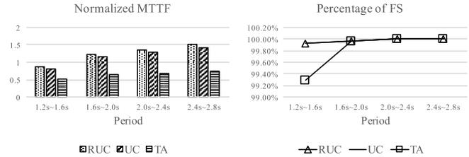
Fig. 11. Normalized MTTF and percentage of FS when tasks' periods are random and running on a TK1-based simulator.
