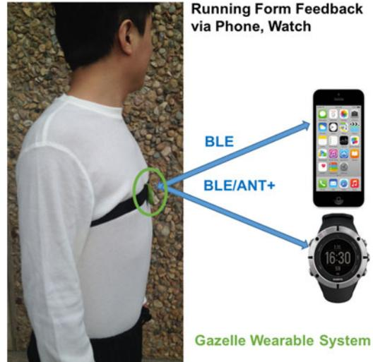
Fig. 3. The example chest worn usage scenario of the Gazelle mobile running analysis system.
