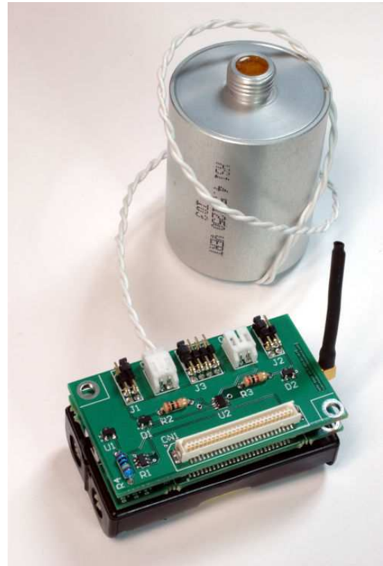
Figure 1: Geophone connected to Mote-Wake board mated to Crossbow Mote
