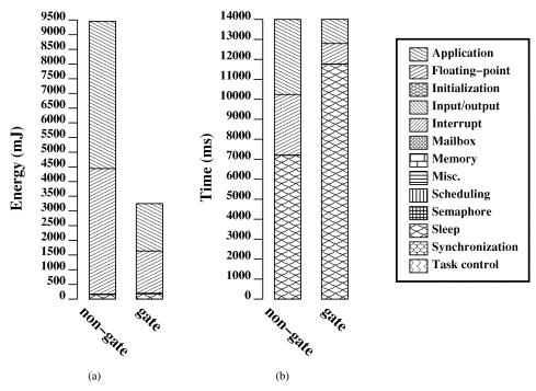
Fig. 2. ABS example: (a) energy and (b) execution time consumption by RTOS service category.
