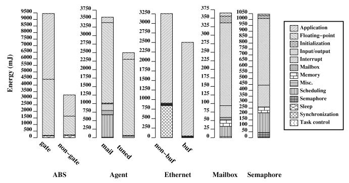
Fig. 9. Energy consumption profiles.
