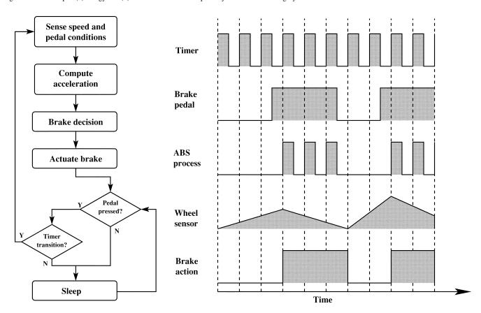
Fig. 3. Energy-optimized implementation of the ABS example.
