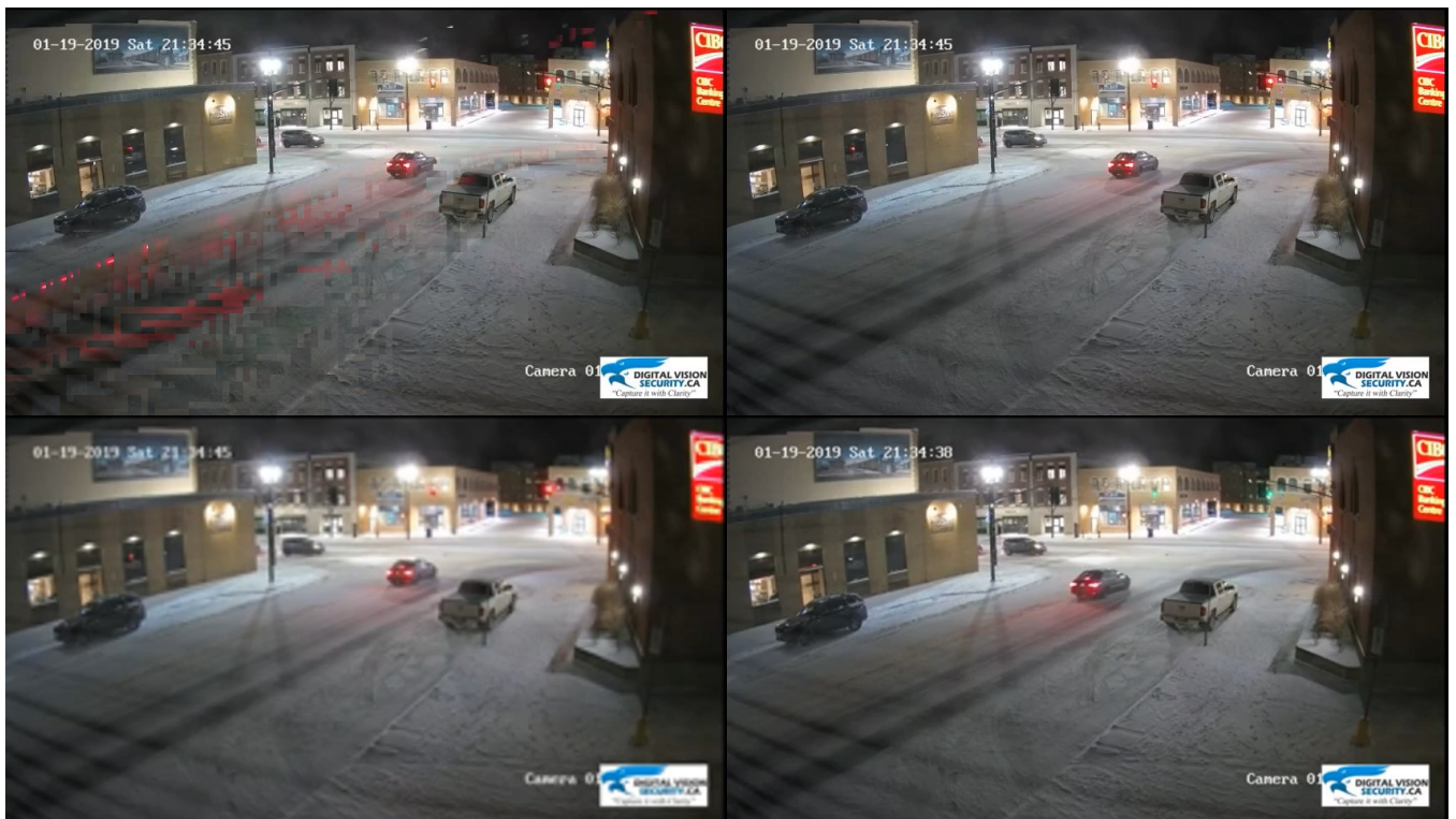
Figure 11: DVS “night” results, clock-wise, starting from top-left: scene cache with parameters determined in section 4.1, original video, uniform downsampling of 31% (bottom-right) and 9% (bottom-left)
