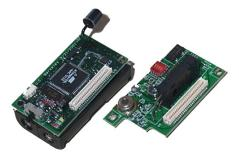
Figure 18.2 Mica mote (left) with Mica Weather Board sensor board for habitat monitoring includes sensors for light, temperature, humidity, pressure, and infrared radiation.
