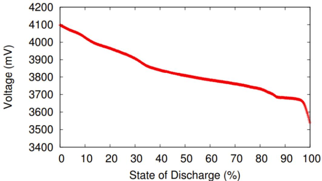
Figure: Discharge curve of ADP2 lithium-ion battery
