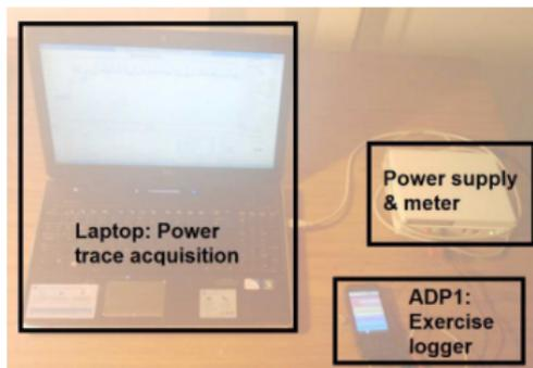
Figure: Experimental setup for power measurement
