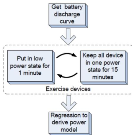
Figure: Battery SOD based power model construction
