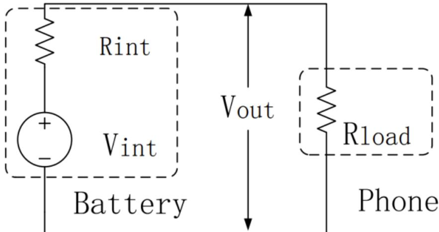
Figure: Equivalent Circuit for Battery
