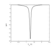
Can find gain by taking  $\sigma V_{out}/\sigma V_{in}$  at  $V_{M}$ .
