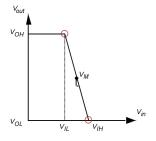
$$V_{IH} - V_{IL} = -\frac{V_{OH} - V_{OL}}{g} = \frac{-V_{DD}}{g}$$
