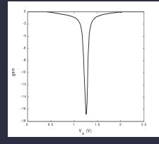
Can find gain by taking  $\sigma V_{out} / \sigma V_{in} \text{ at } V_M.$   $g = -\frac{1}{I_D(V_M)} \frac{k_n V_{DSATn} + k_p V_{DSATp}}{\lambda_n - \lambda_p}$ (1)  $g \approx \frac{1}{\left(V_M - V_{Tn} - \frac{V_{DSATn}}{2}\right)(\lambda_n - \lambda_p)}$ (2)
