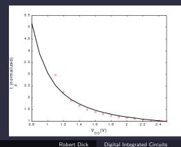
Dependence of inverter delay on  $V_{DD}$  I
