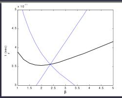
$\beta = W_{P}/W_{n}.$   $t_{p} = \frac{t_{pLH} + t_{pHL}}{2}.$
