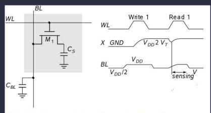
Write: C<sub>S</sub> is charged or discharged by asserting WL and BL.
