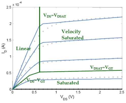
$$\begin{split} I_D &= 0 \ \text{ for } \ V_{GT} \leq 0 \\ I_D &= k' \frac{W}{L} \Big( V_{GT} V_{min} - \frac{V_{min}^2}{2} \Big) (1 + \lambda V_{DS}) \ \text{for } V_{GT} \geq 0 \\ \text{with } \ V_{min} &= \min(V_{GT}, V_{DS}, V_{DSAT}), \\ V_{GT} &= V_{GS} - V_T, \\ \text{and } \ V_T &= V_{T0} + \gamma (\sqrt{|-2\phi_F|} + V_{SB}| - \sqrt{|-2\phi_F|}) \end{split}$$
