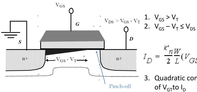
$$I_D = \frac{k'_n \underline{W}}{2} (V_{GS} - V_T)^2 (1 + \lambda V_{DS})$$
