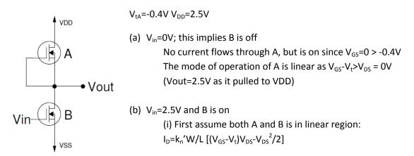
Setting two current in two devices equal:
