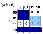
Irredundant but not minimal REDUCE EXPAND IRREDUNDANT
