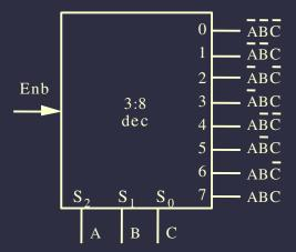
Generate minterm based on control signals
