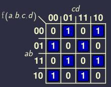
Consider a 4-term XOR (parity) gate:  $a \oplus b \oplus c \oplus d$  $(\overline{a} \ \overline{b} \ \overline{c} d) + (\overline{a} \ \overline{b} \ c \ \overline{d}) + (\overline{a} \ b \ \overline{c} \ \overline{d}) + (\overline{a} \ b \ c \ d) + (a \ b \ \overline{c} \ d) + (a \ \overline{b} \ \overline{c} \ d) + (a \ \overline{c} \ \overline{c} \ d) + (a \ \overline{c} \ \overline{c} \ d) + (a \ \overline{c} \ \overline{c$
