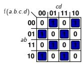
Consider a 4-term XOR (parity) gate:  $a \oplus b \oplus c \oplus d$   $(\overline{a} \, \overline{b} \, \overline{c} \, d) + (\overline{a} \, \overline{b} \, \overline{c} \, \overline{d}) + (\overline{a} \, b \overline{c} \, \overline{d}) + (\overline{a} \, b \overline{c} \, \overline{d}) + (ab\overline{c} \, d) + (ab\overline{c} \, d) + (ab\overline{c} \, \overline{d}) + (ab\overline{c} \, \overline{d}) + (ab\overline{c} \, \overline{d})$
