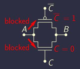
AND and OR are harder than NAND and NOR Transmission gates
