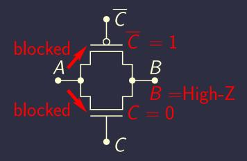
AND and OR are harder than NAND and NOR Transmission gates
