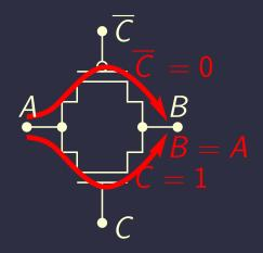
AND and OR are harder than NAND and NOR Transmission gates
