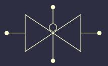
AND and OR are harder than NAND and NOR Transmission gates
